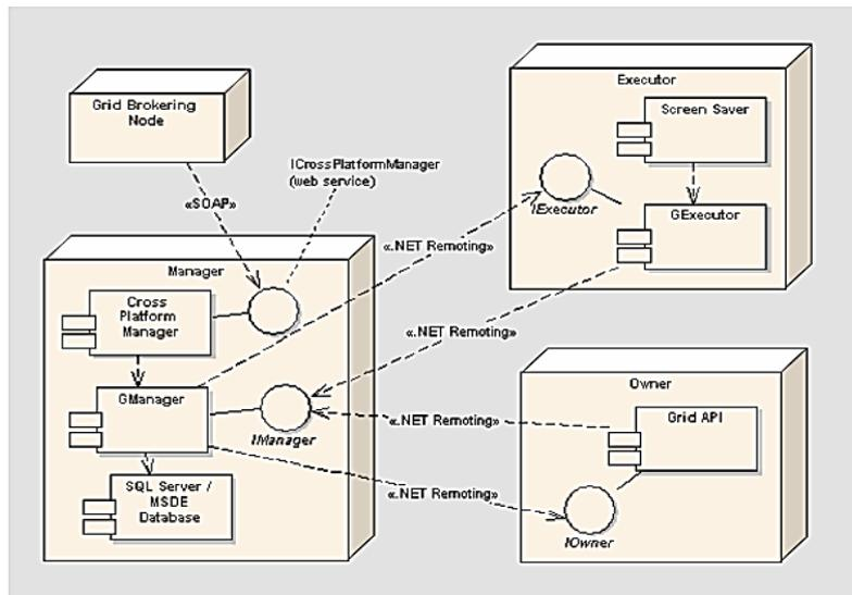
Figure 4. Alchemi architecture and interaction between its components.
