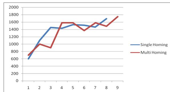
Figure: 14 (End-to-End Delay vs no. of nodes - AOMDV)
