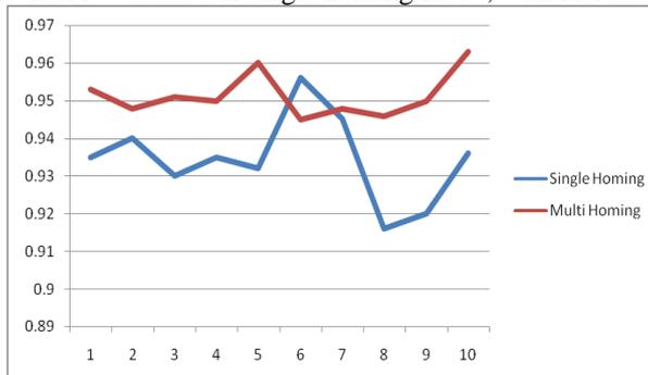
Figure: 4 (Packet Delivery Ratio vs Pause Time – AODV)
