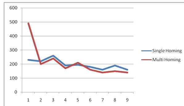
Figure: 9 (Throughput vs no. of nodes – AOMDV)
