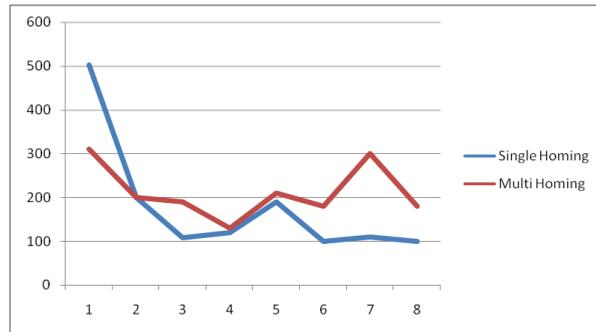
Figure: 7 (Throughput vs no. of nodes – AODV)
