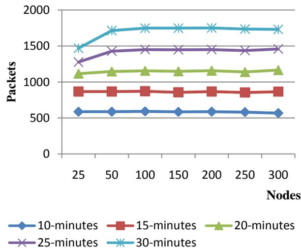
Fig. 4 (a) Packets delivered versus network size with mobility for different Simulation time
