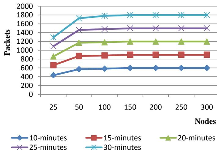
Fig. 4 (b) Packets delivered versus network size without mobility for different Simulation time
