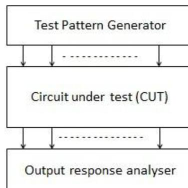
Fig1. Block Diagram for BIST
