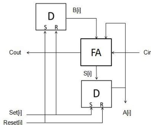
Fig 2. Accumulator cell
