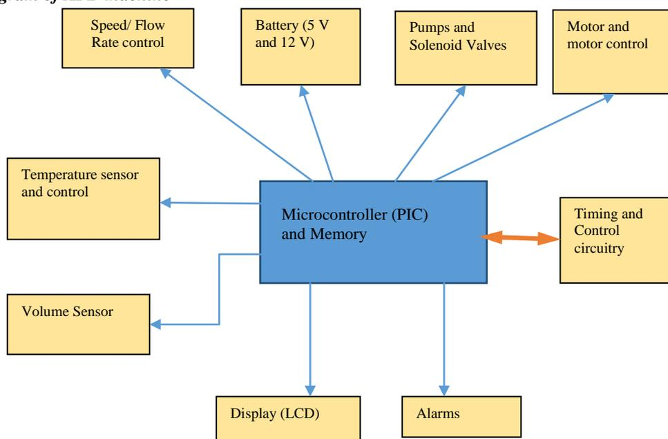
Figure (4): Block Diagram of the Proposed Model
