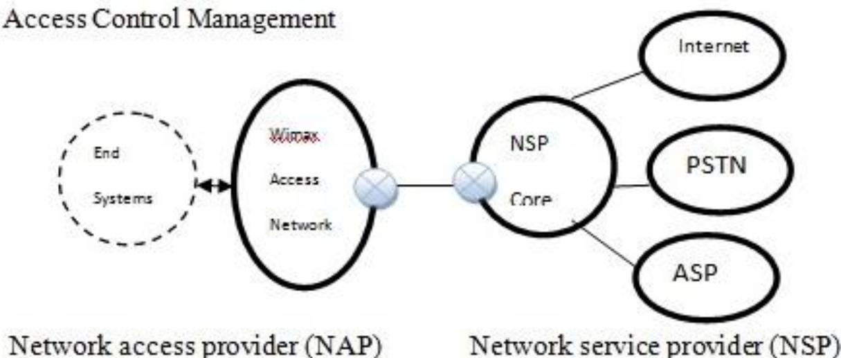
Figure 2: Mobile WiMax architecture
