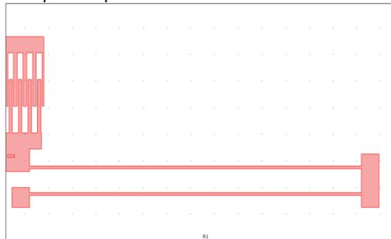
Figure 1.4: Actuator with  $1\mu\text{m}$  Spacing and 4 Moving Combs.
