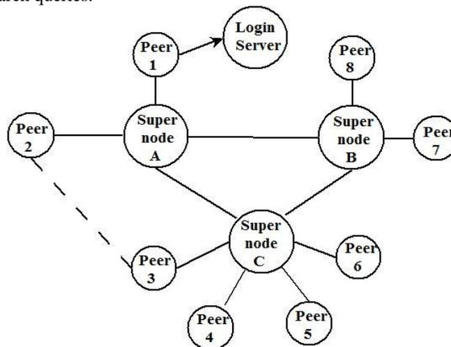
Figure 3. Notational instance of Skype architecture.
