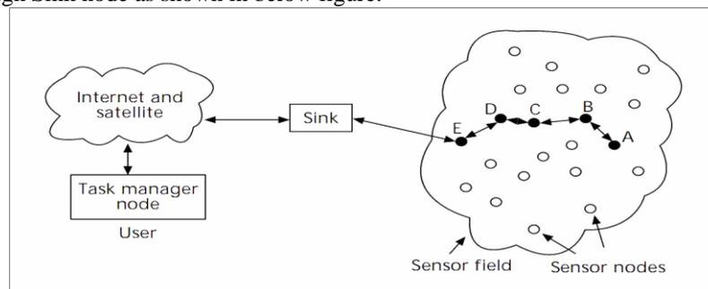
Fig 1 Sensor nodes scattered in a sensor field
