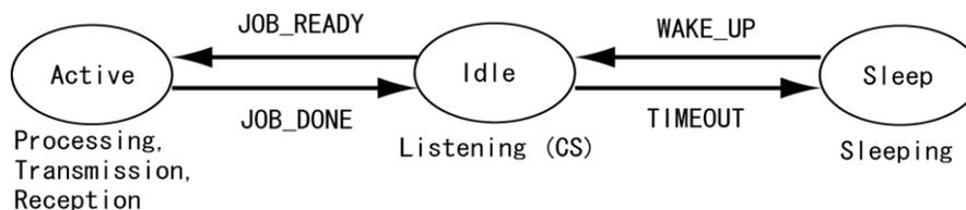
Fig 4 A State Diagram of Sensor Node
