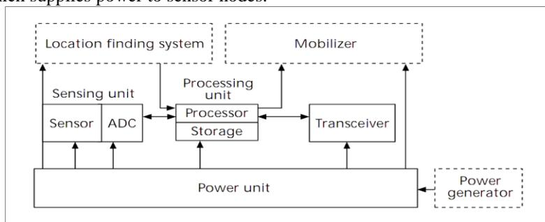
Fig3 Components of Sensor Node
