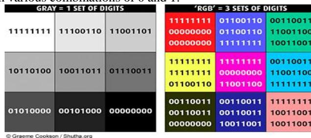
Fig.4 A greyscale image only has 1 set of numbers per pixel, an RGB image has three sets of numbers per pixel and a CMYK image has four sets of numbers per pixel
