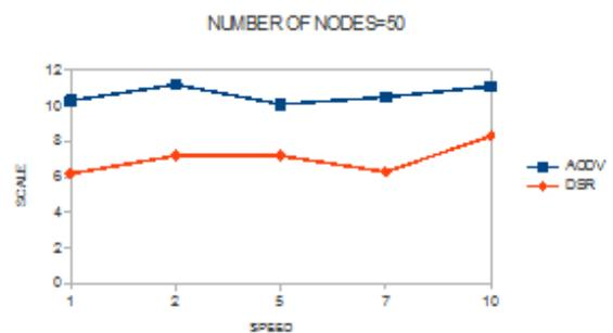
Fig. 6 Reliability on speed for 50 nodes
