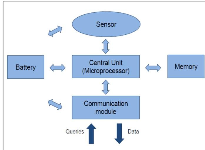
Fig. 2 Architecture of a sensor node
