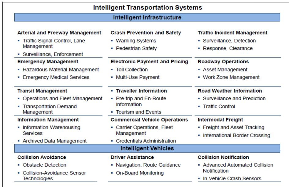
Fig. 4 Overview of ITS applications and examples
