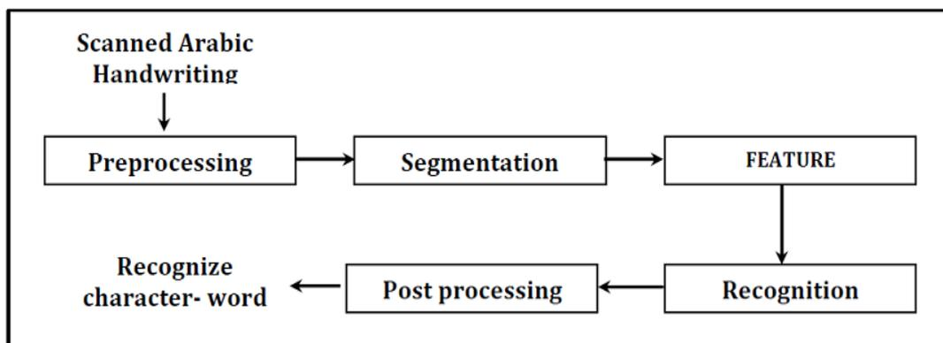
Figure 5: A typical OCR system
