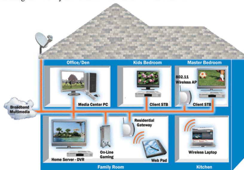
Structure of Networking between the different computers
