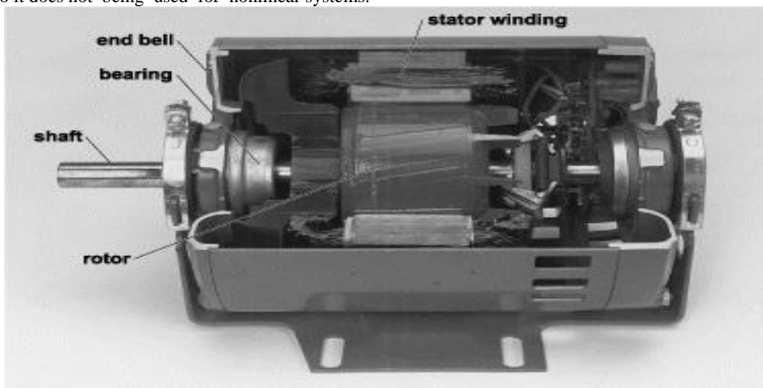
Fig 1.1 Cut View of Induction Motor
