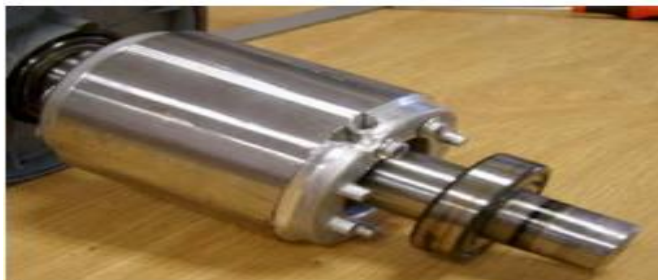
Fig.1.5 Cast Rotor of Induction Motor
