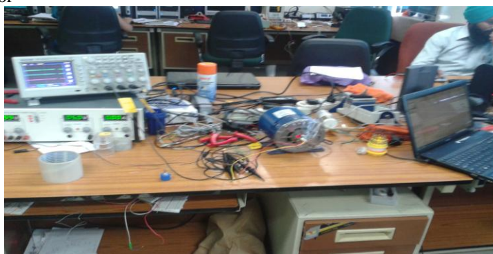
Fig.4 Test bench for Vibration condition monitoring
