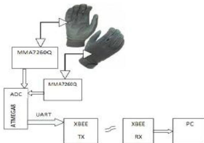
Figure 5: General Data Flow of the Circuit
