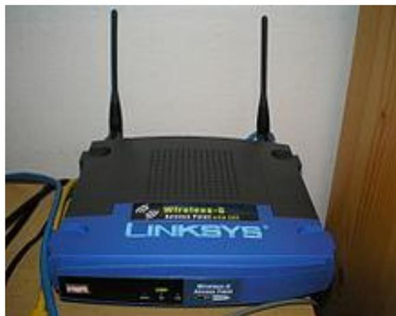
Fig3 Linksys Mobile "WAP54G" 802.11g wireless Access Point
