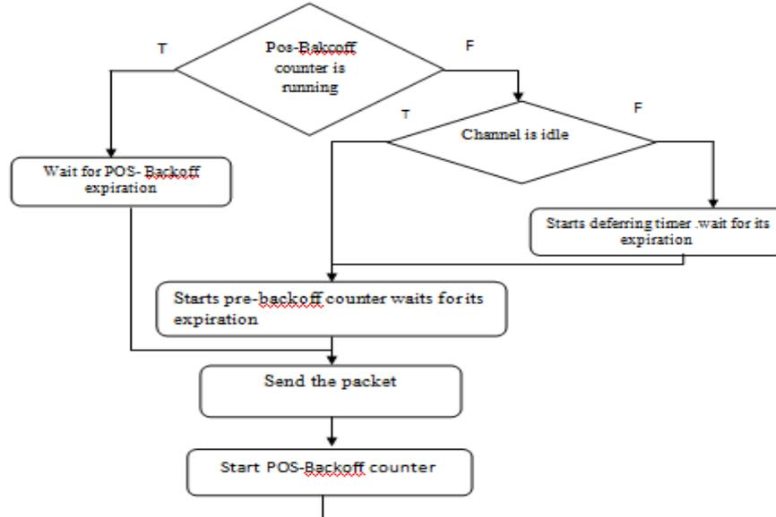
Figure 1: IEEE 802.11 MAC Algorithm To Transmit A Frame.[7]
