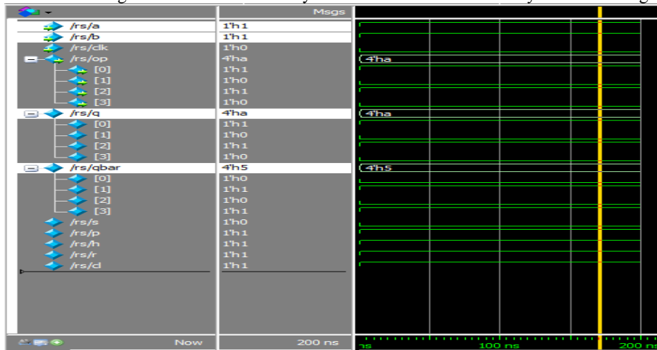
Fig. 3 Simulation output for SIPO shift register of 4 bit input data.
