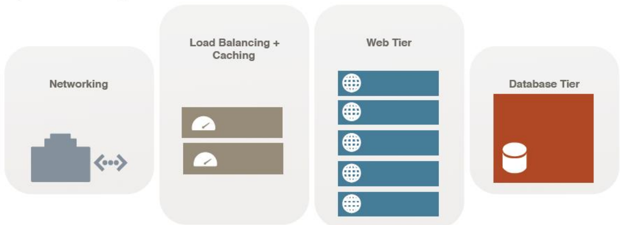
Figure 2: Horizontally scaled load balancing and web-tier. Vertically scaled database tier.
