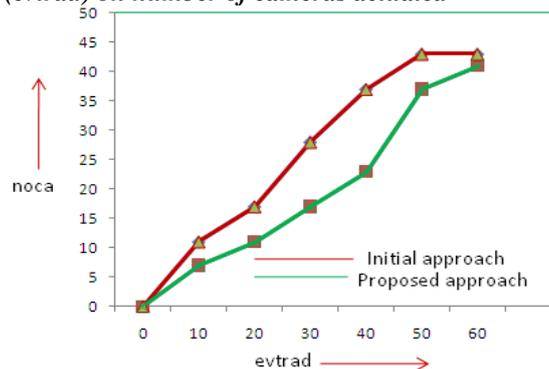
Fig. 5 Effect of varying event radius (evtrad) on number of cameras actuated
