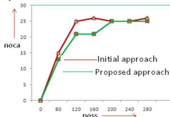
Fig. 2 Effect of varying number of scalars (noss) on number of cameras actuated (noca)
