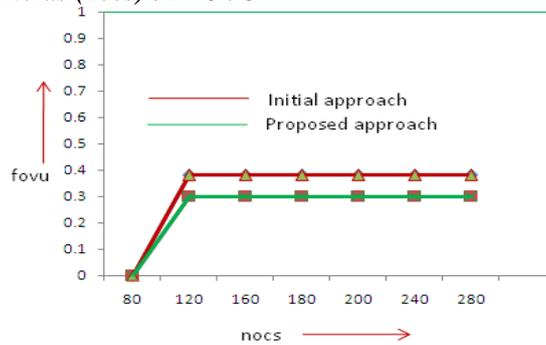
Fig. 7 Effect of varying number of cameras (nocs) on Field of view utilization (FOVU)
