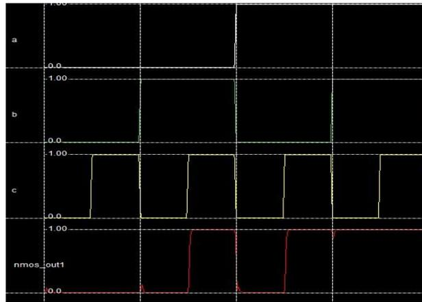
Figure 10 Waveform of Carry for Proposed Adder
