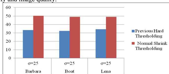
Fig. 1 Comparison of Hard Thresholding and Normal Shrink Thresholding
