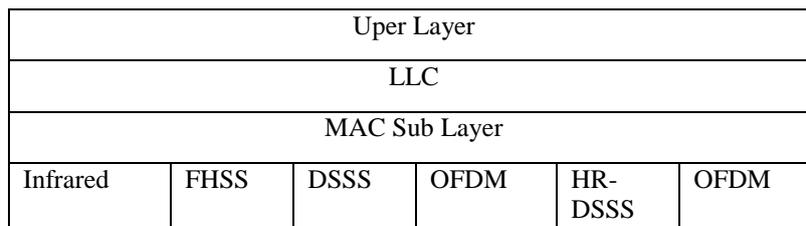
Figure 3 Layer Protocol Stack
