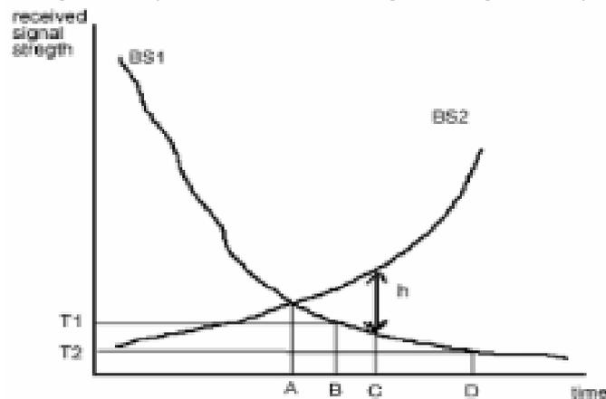
Fig.1 Movement of an MS in the handoff zone
