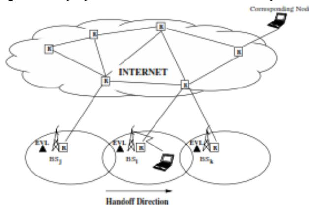
Fig..3 An illustration of wireless environment during handoff of mobile station from BS<sub>1</sub> to BS<sub>2</sub>.
