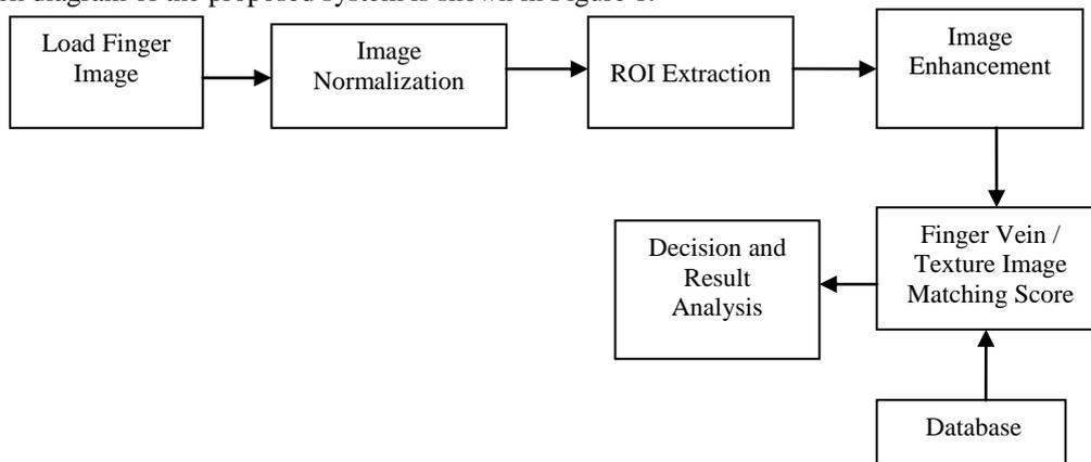
FIGURE 1: DIAGRAM OF PROPOSED SYSTEM
