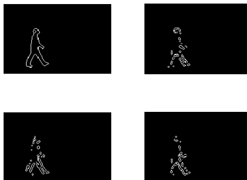
Figure 3.2: Canny edge detected wavelet coefficients
