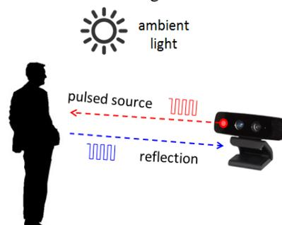
Figure 1: TOF (Time of Flight) technique for depth
