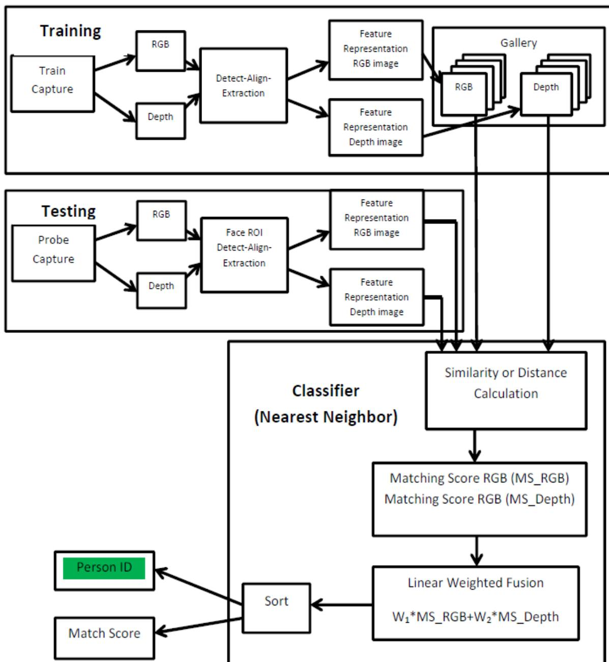
Figure 2: System Functional Diagram for RGB-D Face Recognition
