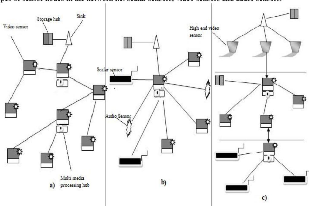
Figure 2. Network architecture for WMSNs
