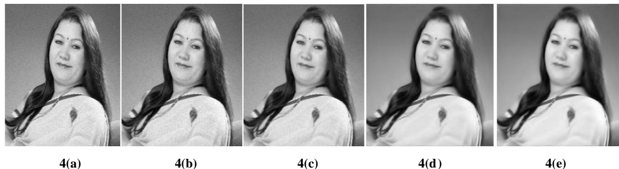
Fig 4: Denoising of ‘Chhaya’ image corrupted by Poisson noise (a) noisy image (b) median filter (c) wiener filter (d) hard thresholding (e) proposed method
