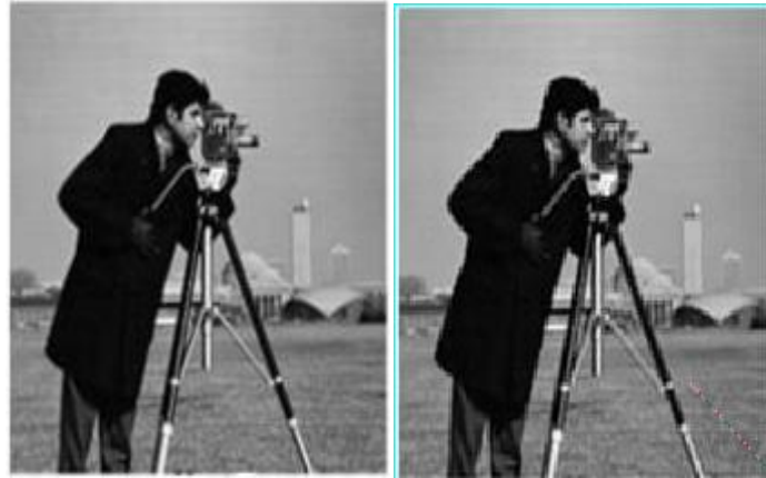
Cover Image(1) Stego Image(2) PSNR between Image (1) and Image (2) = 118.38 MSE between Image (1) and Image (2) = 0.078
