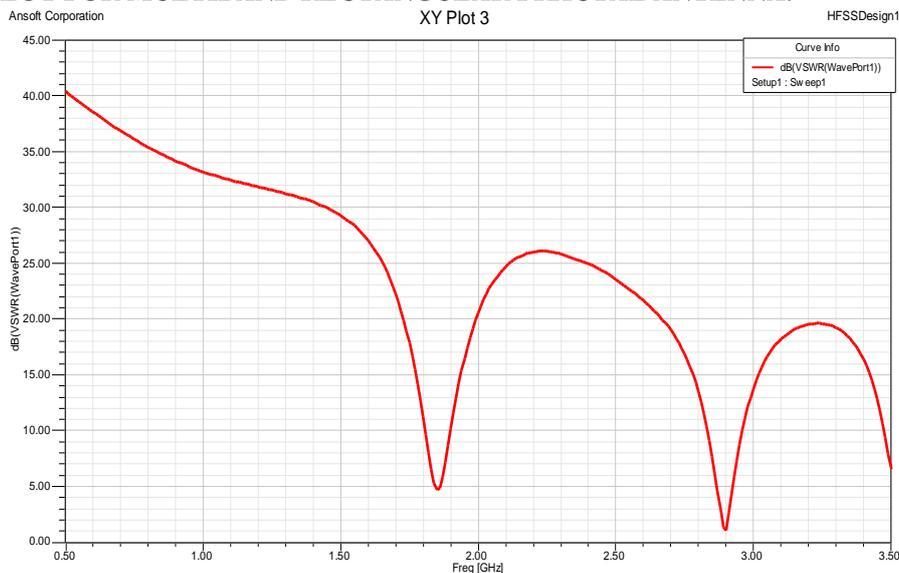
Fig. 4.2: VSWR plot for Multiband Rectangular fractal antenna.
