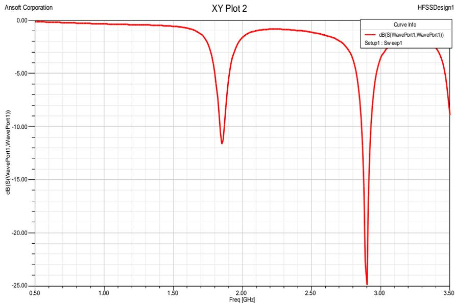
Fig. 4.1: Return Loss plot for multiband rectangular fractal antenna.
