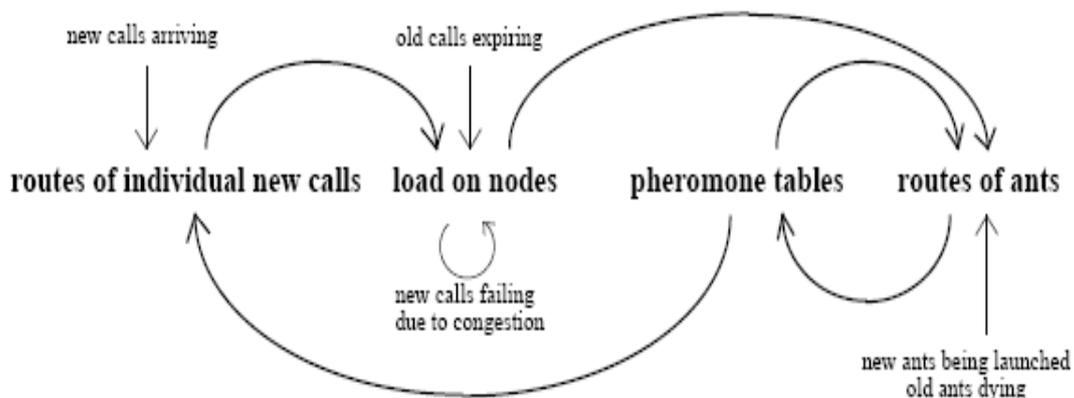
Fig. 3.1 Figure 3 Relationship between calls, node utilization, pheromone tables and ants. An arrow indicates the direction of influence [16].
