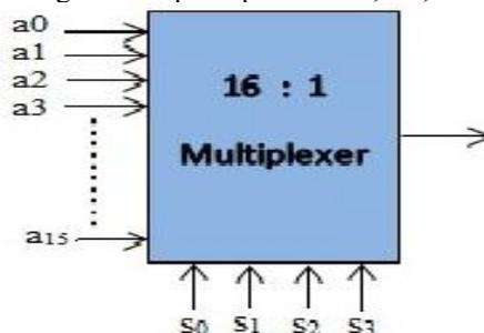
Fig (6): Block diagram of 16:1 multiplexer containing designs for alphabet 'a'.
