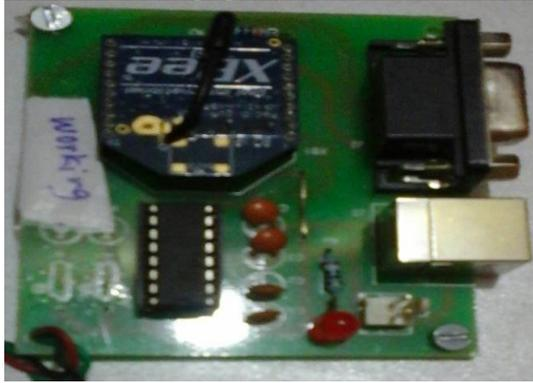
**Figure 4: Zigbee Transmitter**
