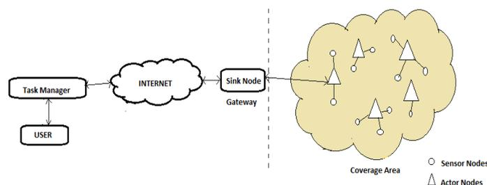
Fig 1: Architecture of Wireless Sensor and Actor Networks
