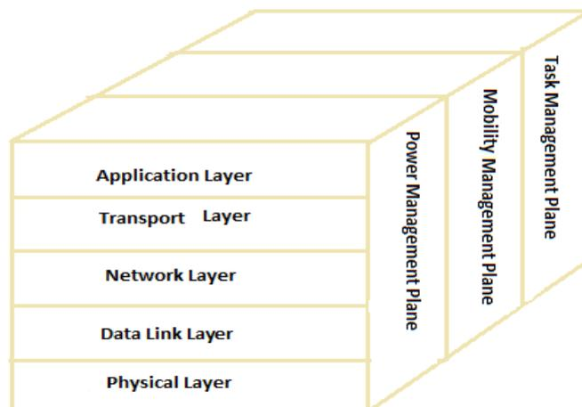
Fig 4: Layered Architecture of WSN
