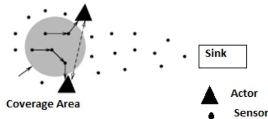
Fig 2: Semi-Automated Architecture
