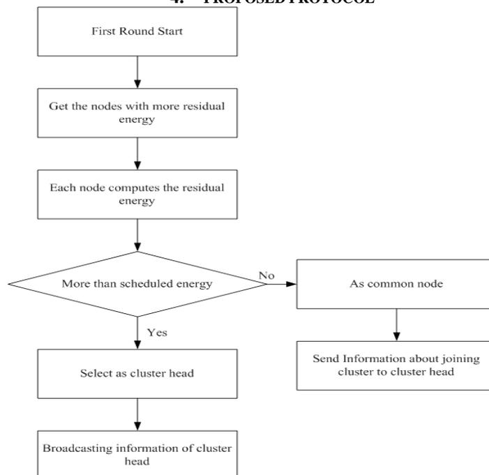
Figure 5: Flow chart of energy modified LEACH proposed protocol [11].
