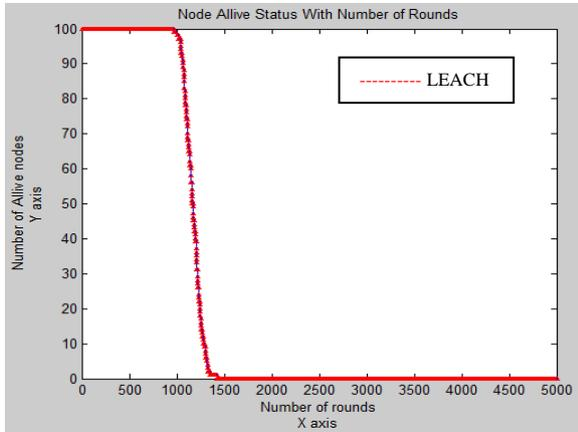
Figure 9: Showing the number of alive nodes vs. number of rounds in a network using the LEACH protocol. The number of nodes is 100
