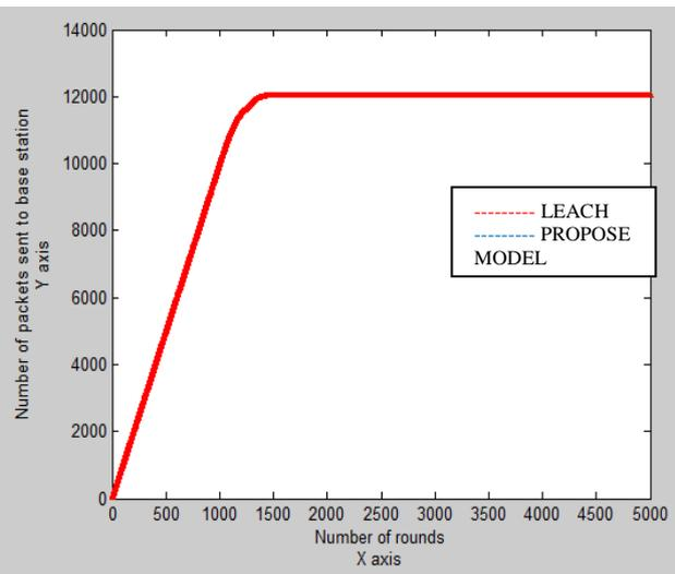
Figure 12: Accumulated number of packets sent to base station vs the number of rounds in the typical network with 100 nodes, 100m x and 100m y area.
