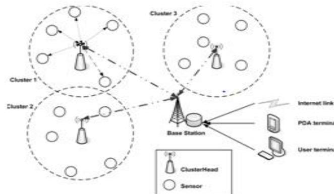
Figure 1: wireless sensor network architecture [1].
