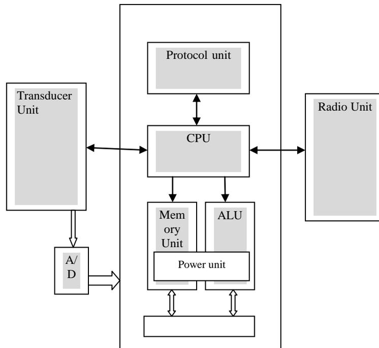
Figure 2: Functional components of a typical WSN.
