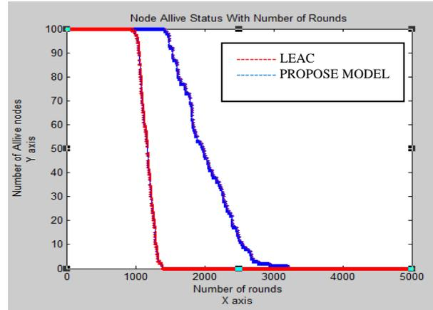
Figure 10: Showing the number of alive nodes vs. Number of rounds in a network with 100 nodes, 100m x and 100m y area.
