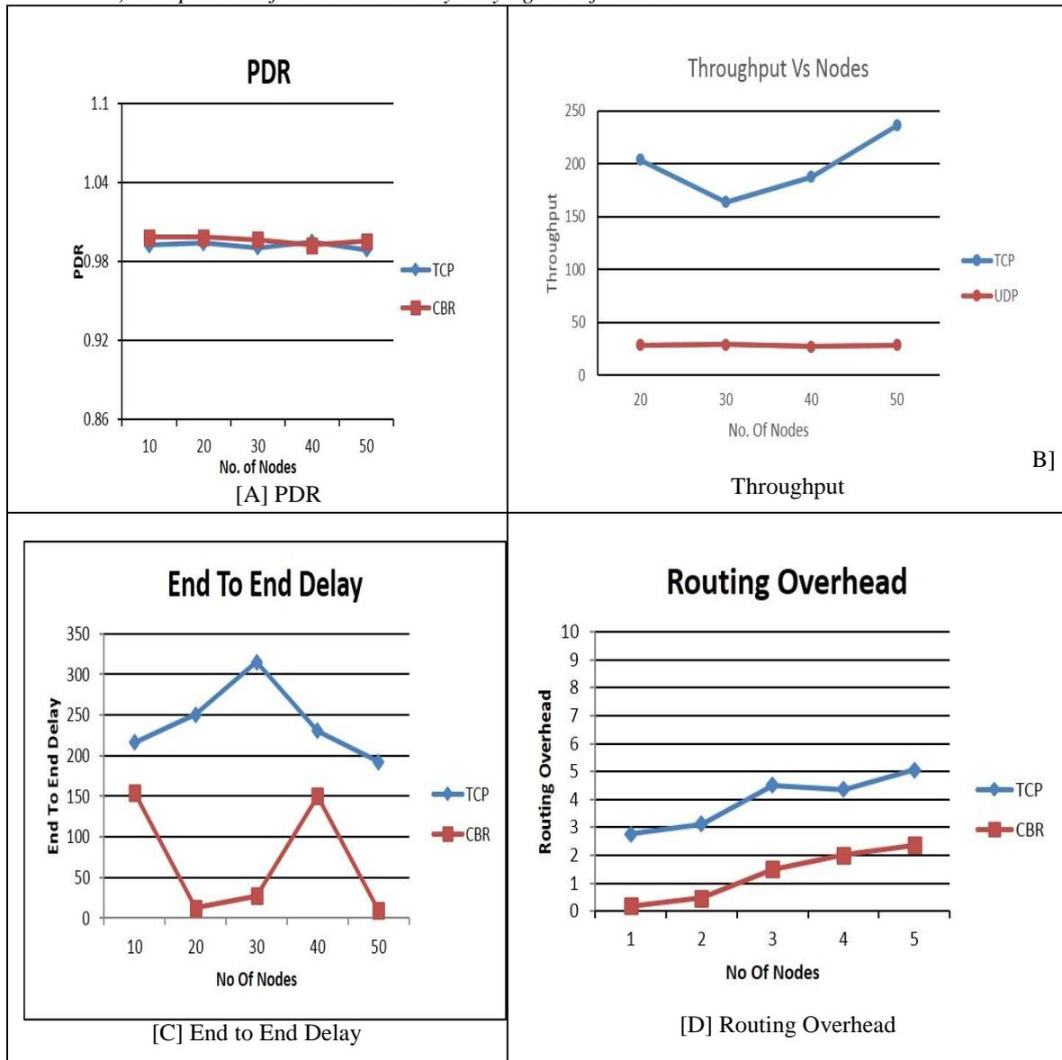
Fig 3 Comparison of PDR, Throughput, Routing Overhead and End to End Delay by varying No of Nodes
