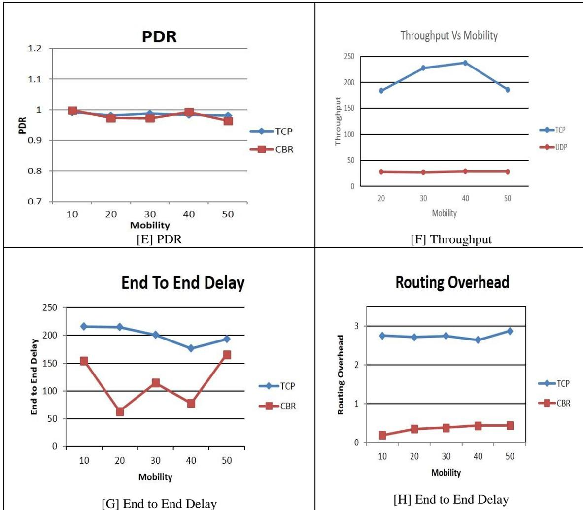
Fig 4 Comparison of PDR, Throughput, Routing Overhead and End to End Delay by varying Mobility
