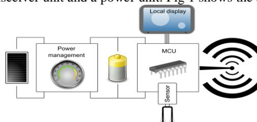
Fig. 1 Architecture of a wireless sensor node
