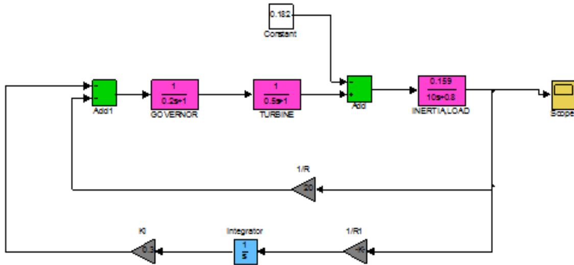
Fig. 3.1 Close loop AGC system for single area
