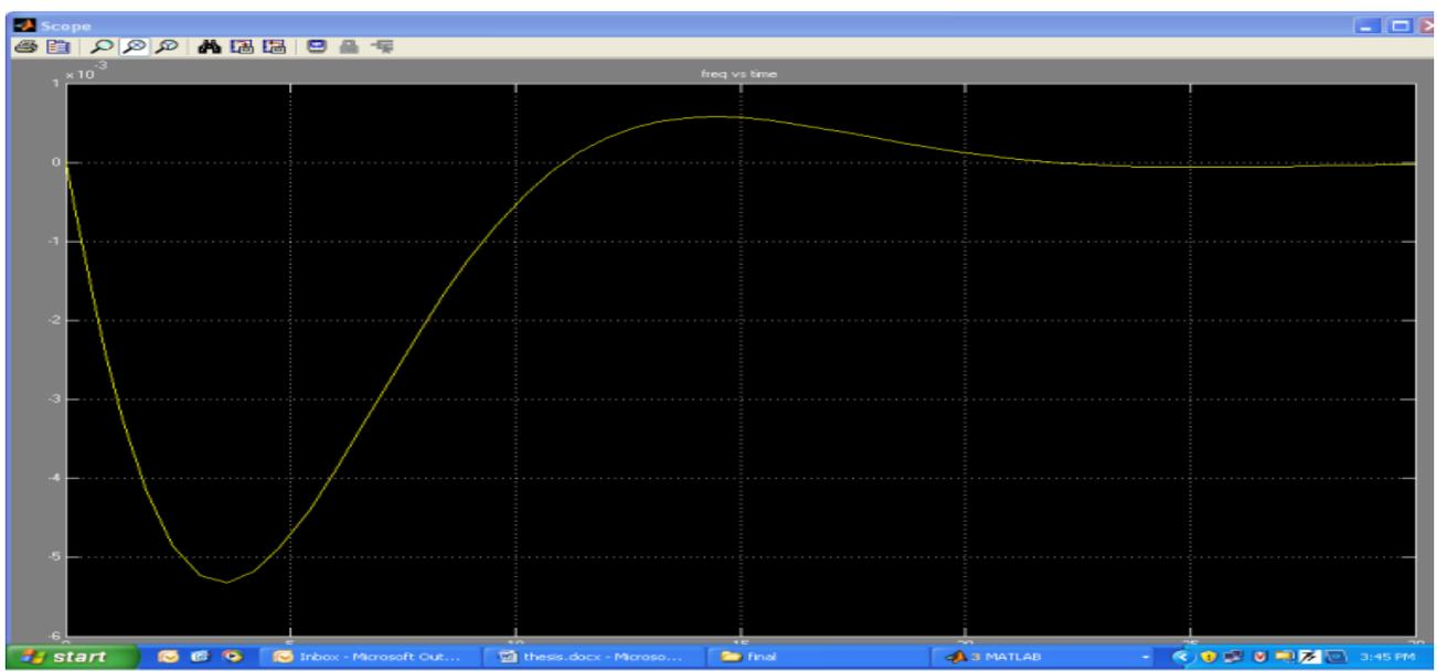
Fig. 3.2 Response for close loop AGC system
