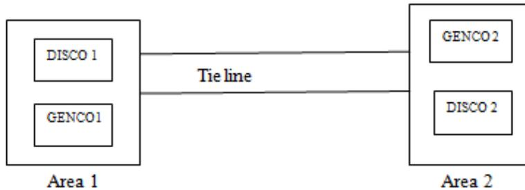
Fig. 3.4 Schematic of a 2 area system in restructured environment
