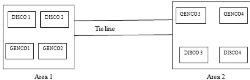
Fig. 3.3 Schematic of a 2 area system in restructured environment
