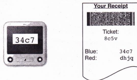
Figure 1-5: A secret receipt in the Neff voter verification scheme - The screen displays a code, which should match the voter's selected option on the receipt. In addition, the ticket number should match the voter's random challenge. Once the voter leaves the booth with only the receipt, it is impossible for her to provably claim that she saw 34c7' on the screen, and not dhjq.
