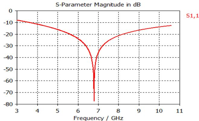
Figure 3: Simulated Return Loss of Tapered Slot Vivaldi Antenna
