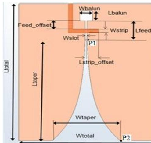
Figure 1: Tapered Slot Vivaldi Antenna
