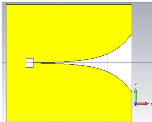
Figure 2(a): Front View of Vivaldi antenna
