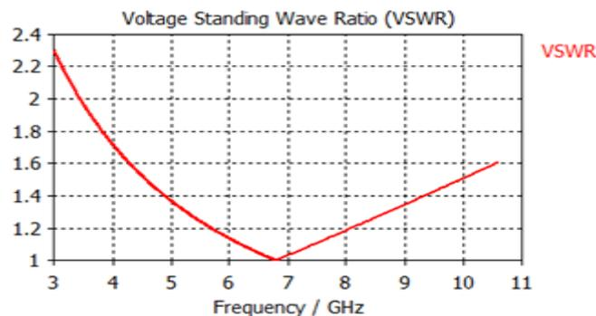
Figure 4: Simulated VSWR of Tapered Slot Vivaldi Antenna
