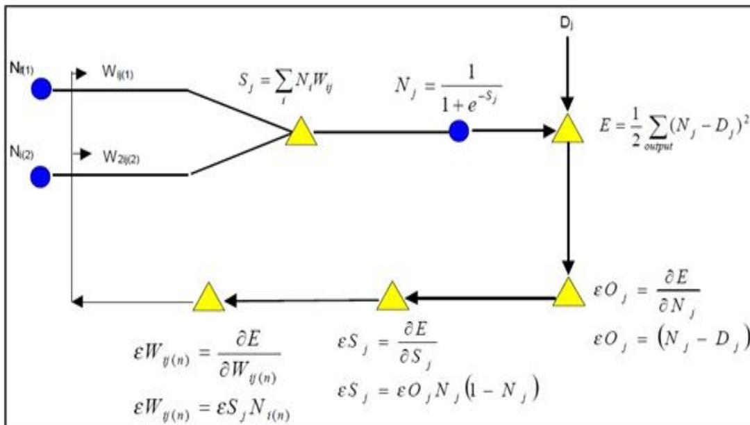
Figure 2 Artificial neural network with backpropagation
