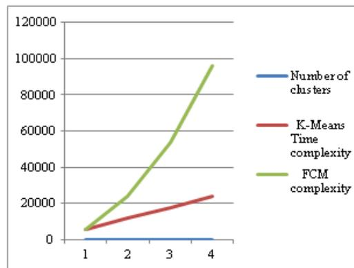
Fig.3. Time complexity of K-Means and FCM by varying number of clusters
