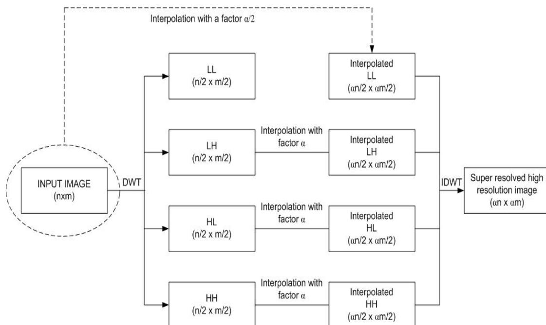
Figure 2: Block diagram of DWT-SR method.
