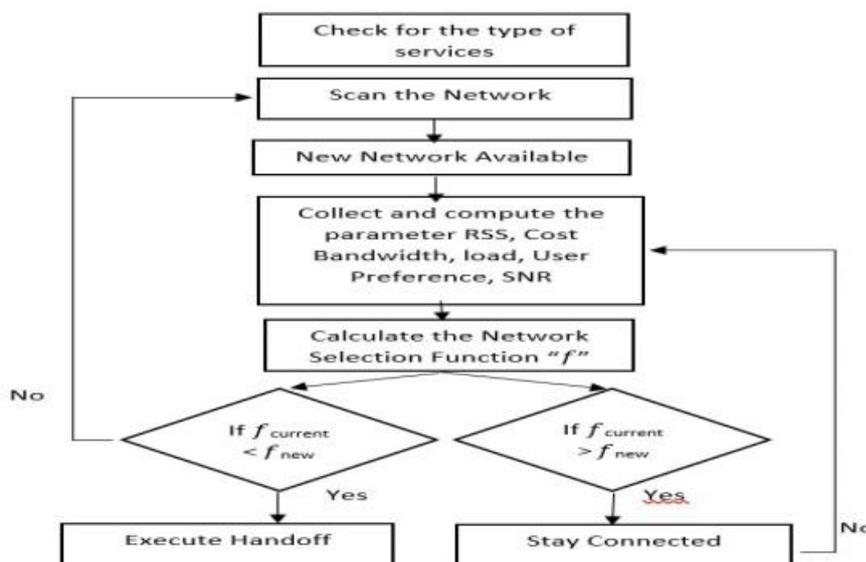
Fig. 5: Mechanism of Network Selection for QoS Based VHO
