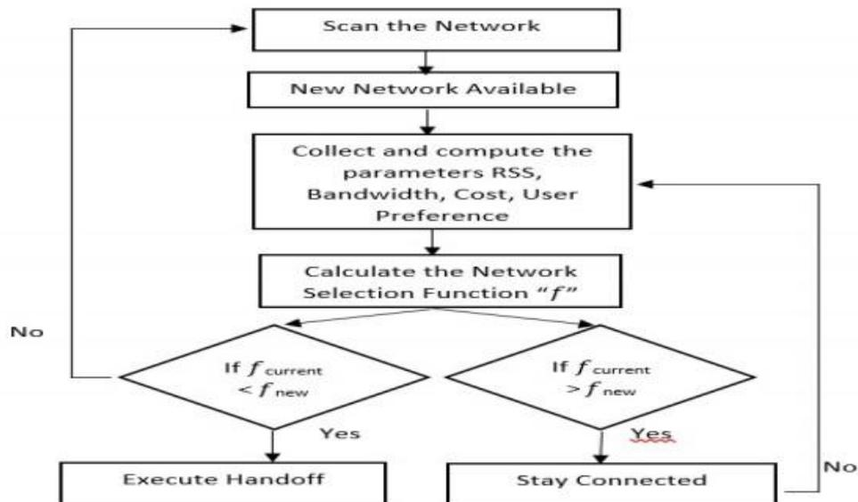
Fig. 3: Mechanism of Network Selection for Cost Function Based VHO
