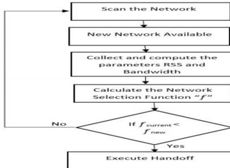
Fig. 2: Mechanism for Network Selection Function for RSS Based VHO
