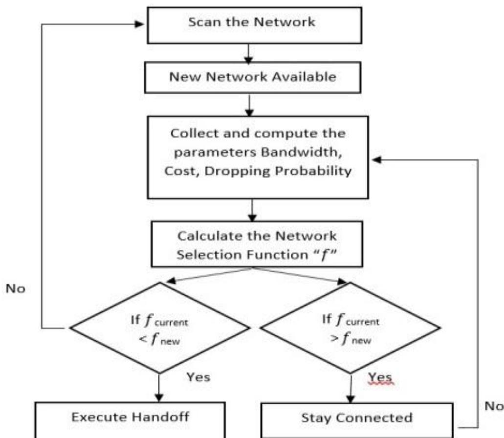
Fig. 4: Mechanism of Network Selection for Processing Delay Based VHO
