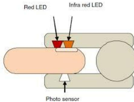
Fig.3 finger inserted in nellcor probe
