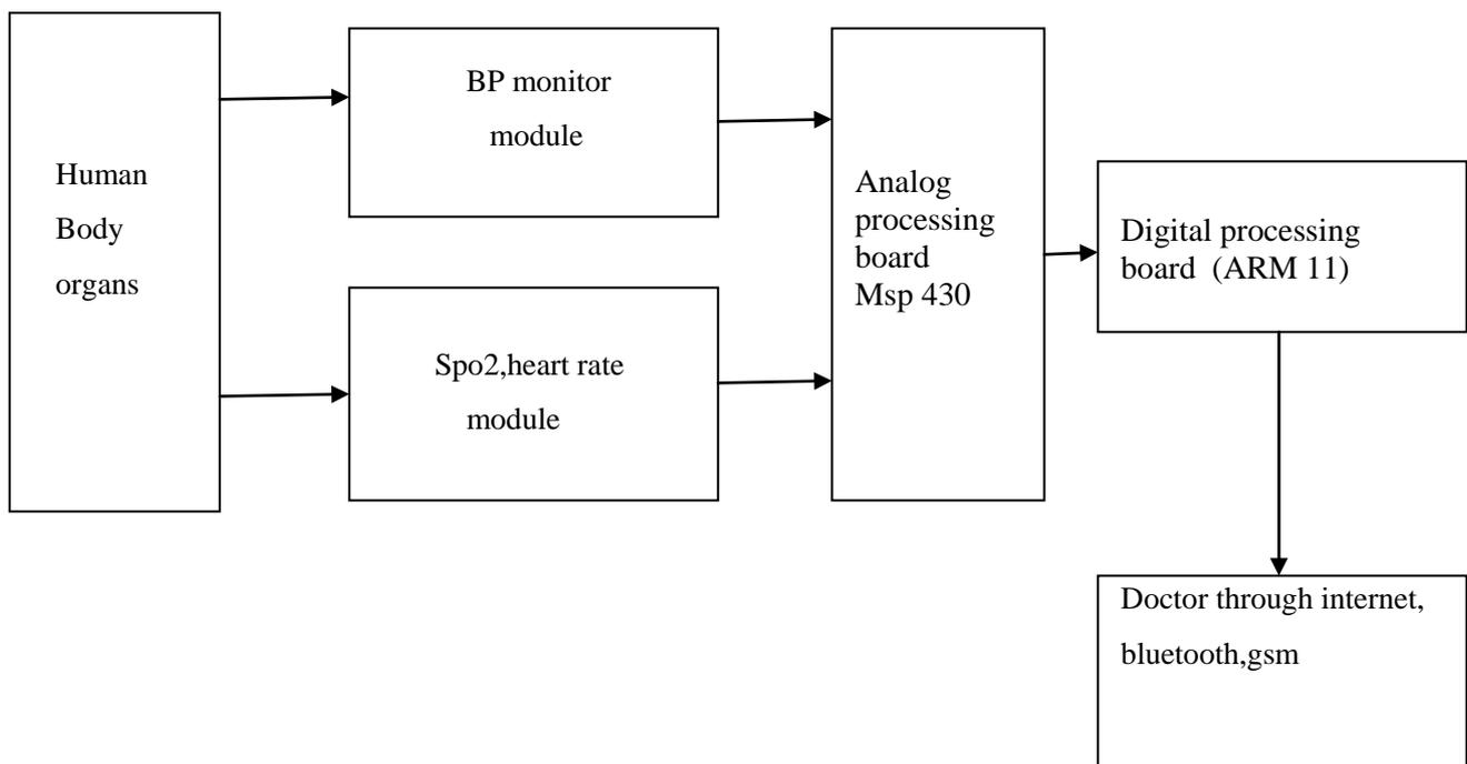
Fig.1 Block diagram of embedded web server for medical field
