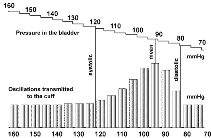
Fig. 7 graph showing principle of systolic vs diastolic BP
