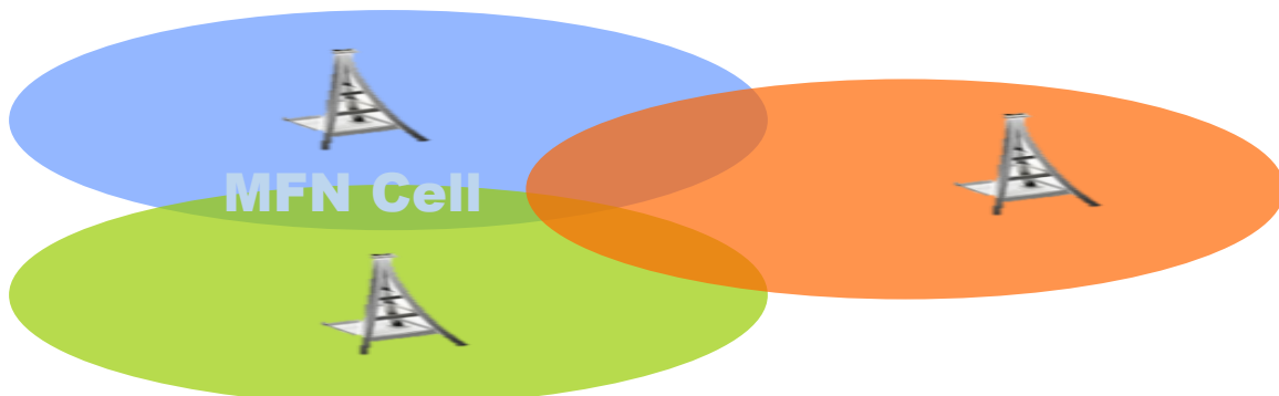
Figure 10: Diagram showing the Multiple Frequency Network (MFN) cell where all transmitters broadcast with different frequencies.
