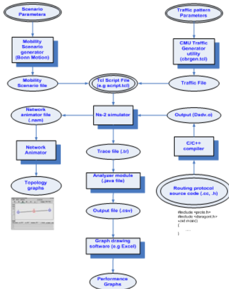
Fig. 1 Flow diagram for evaluating the performance in MANET Routing Protocols
