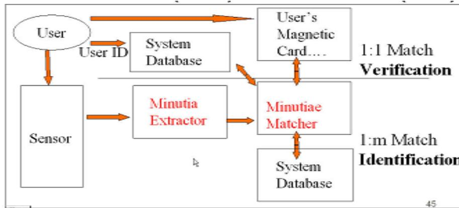
Figure-3: Automatic Finger Recognition System [4].
